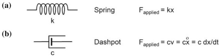
Fig. 4.43 a Ideal (or perfect) spring and b ideal (or perfect) dashpot. These are the two basic building blocks used in modeling the mechanical response of materials
