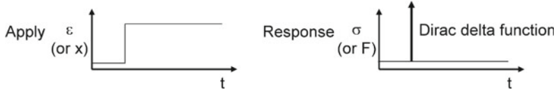
Fig. 4.55 Response by a perfect dashpot. a Creep. b Stress relaxation
