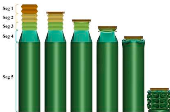
Fig. 27. Deformation mode with a five-stage response.
