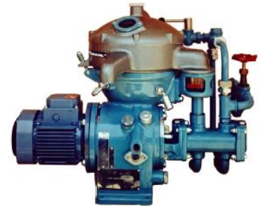
Fig1.MAB 103B-24, with feed and discharge pump.
